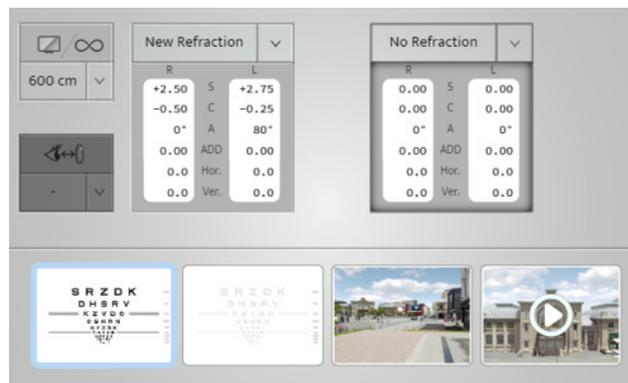
On the initial screen, the default comparison values are [New refraction] and [No refraction]. As you had a lensmeter value in the memory bank, it will automatically have these two comparisons already selected.
