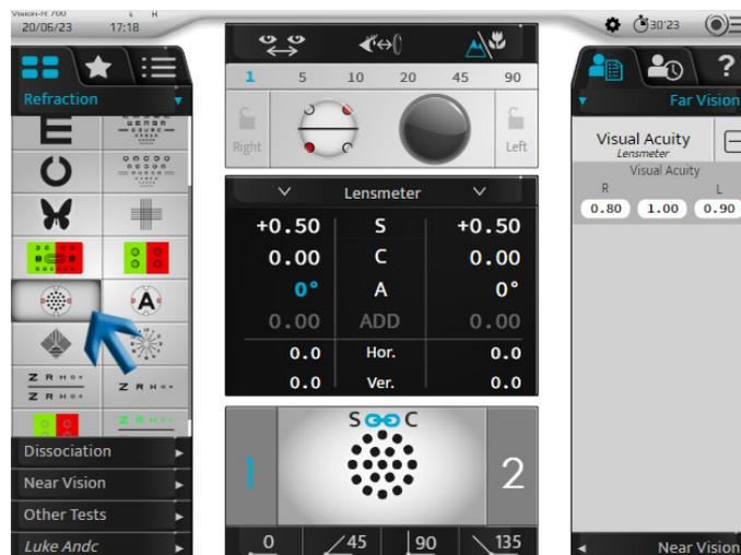
> The dot test is displayed on the test presentation screen.
