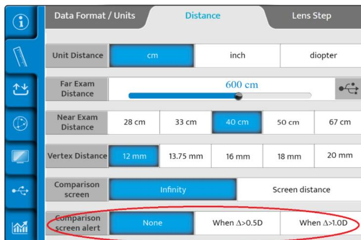
When activated, the ECP can decide whether to see this "Alert" when the dioptric difference is greater than 0.50 D or when greater than 1.00 D.
