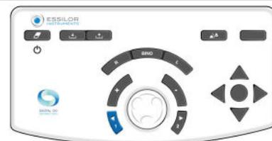
To show the dots in position 2, press the "2" key on the console keyboard.
