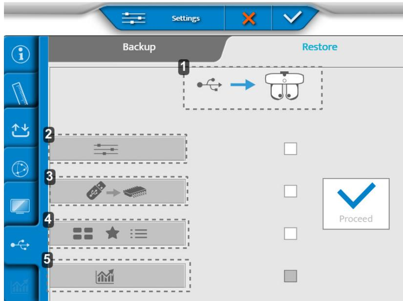
1. *Importing of data from an USB key to the refraction head*
