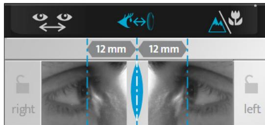
> Adjust the position of the vertical lines to match the corneal apex of each eye using the central button or the incrementation keys (+/-) on the console keyboard.
