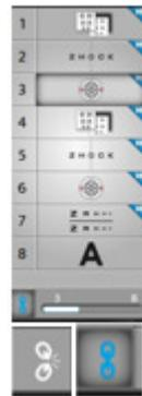
"Auto next" is a feature to help speed up the process and help the ECP to perform less actions. When this feature is activate, the Smart Program will automatically move to the next test and start it immediately. If this feature is deactivated, the program will ask you to initiate the next test once the end point has been calculated in the current test.
